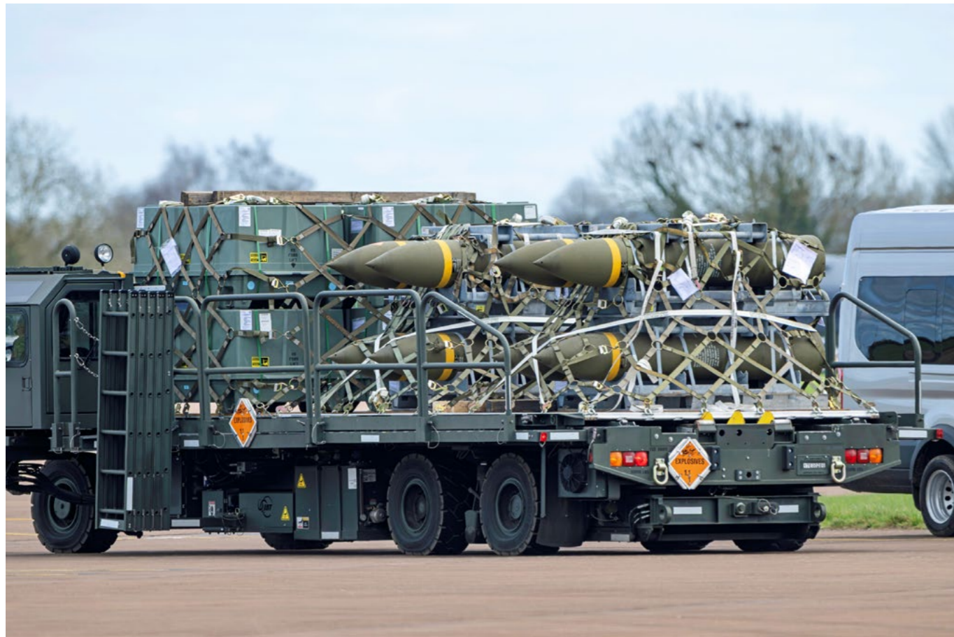
Building the Loadout: A Halvorsen loader transports a fresh supply of BLU-109 bomb bodies and component crates across the RAF Fairford apron. These “iron bombs” serve as the foundation for the precision-guided munitions that define the B-1B Lancer’s conventional strike mission.
