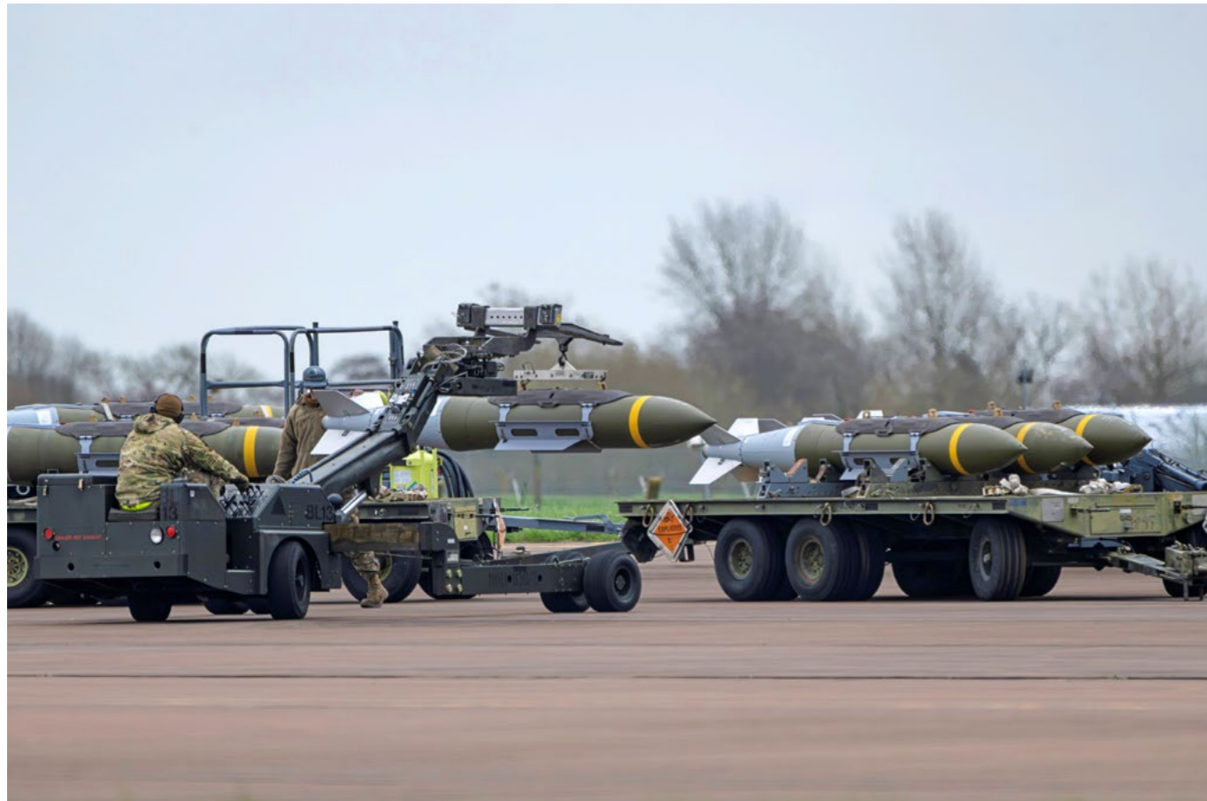
Loading the Bone: Airmen utilize an MJ-1 lift truck to transfer BLU-109 munitions from transport trailers to a B-1B Lancer. This “last mile” of the munitions chain is critical for maintaining the rapid sortie rates required during Operation Epic Fury.
