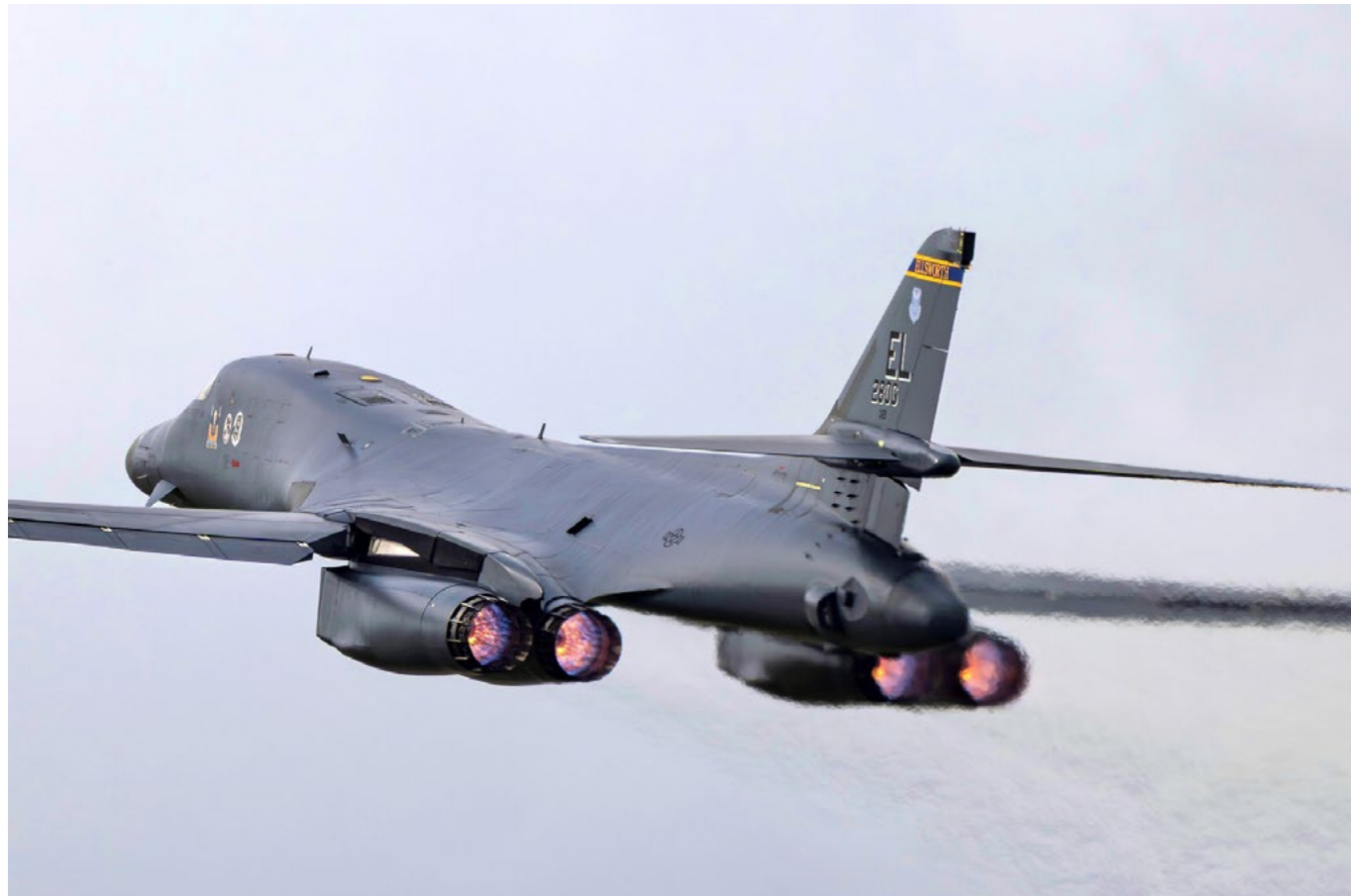
Full Afterburner The raw power of the B-1B Lancer is on full display as it departs Fairford with all four GE F101 engines in afterburner. This "Bone" from the 28th Bomb Wing creates a massive heat signature while climbing out for a long-duration mission.
